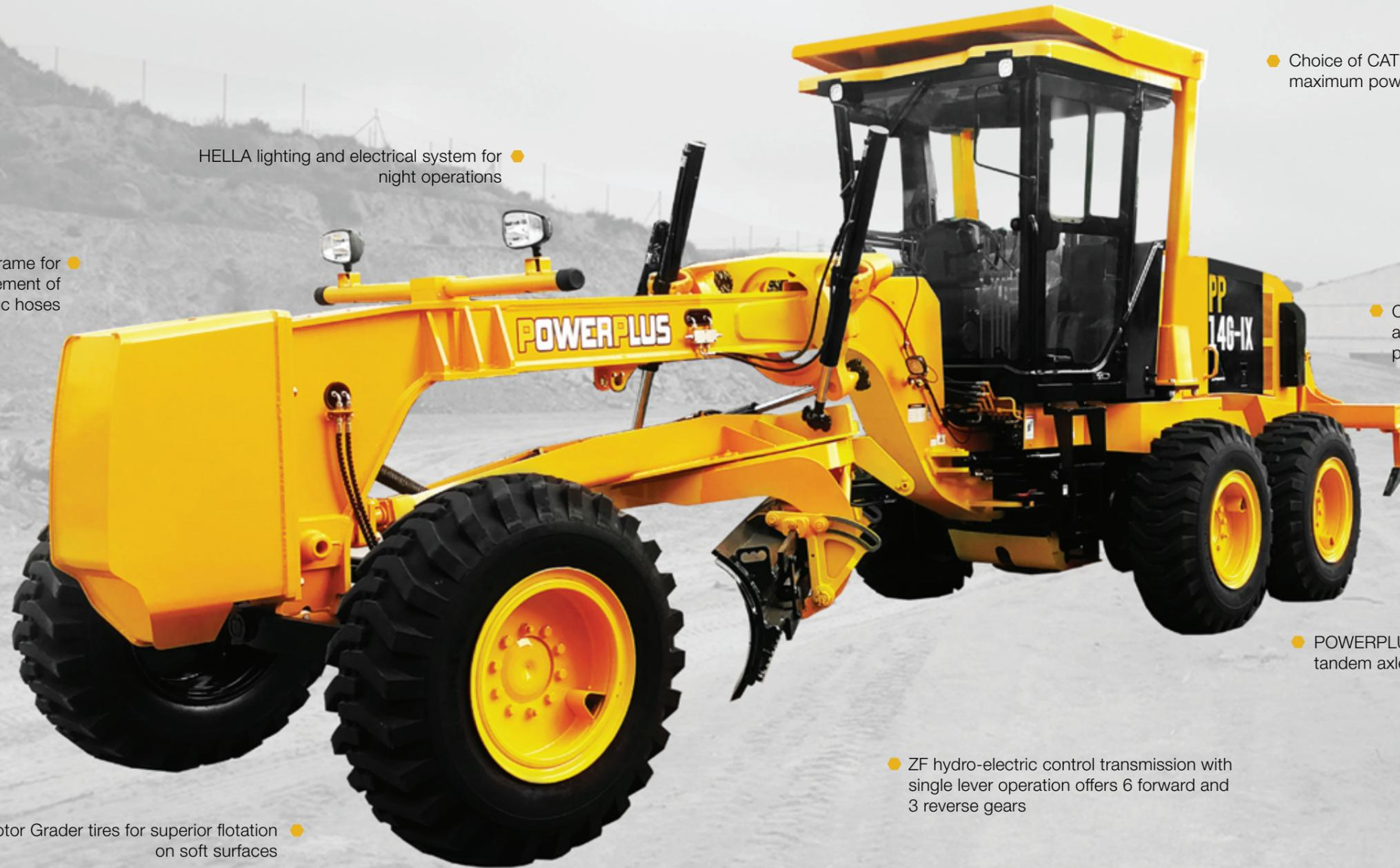
● Ergonomic air-conditioned cabin that reduces external noise and vibration. Excellent visibility of glass cabin boosts operator's confidence and productivity
