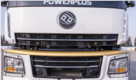
● LIGHTING HID lights secure maximum visibility in harsh weather conditions.
