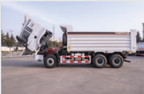
● CABIN Tilttable cabin for convenient inspection and maintenance.
