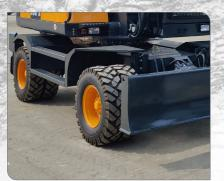
A robust dozer blade & outriggers optimize machine stability and versatility
